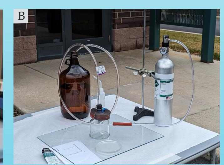
Figure 2. (A.) In-house Cl<sub>2</sub> gas generation and delivery system. Note the Cl<sub>2</sub> concentration was not known during exposures, thus the true dose was not known for this set of experiments. (B.) In-house Cl<sub>2</sub> gas delivery system. Note the Cl<sub>2</sub> concentration was known (1,200 ppm in air), thus the dosage (concentration x time) could be adjusted according to the required experimental conditions.
