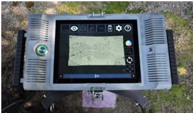
Exhibit 5. Overhead view of touchscreen interface with footwear scan on screen.
