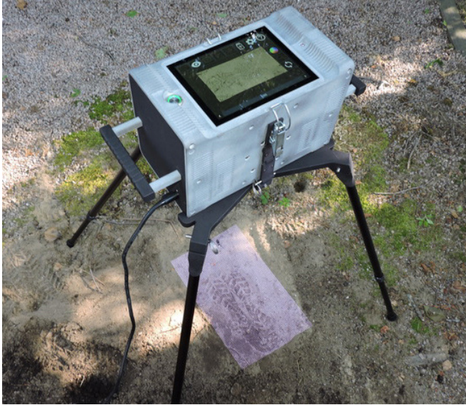
Exhibit 2. 3D scanner set-up to capture a footwear impression in soil.
