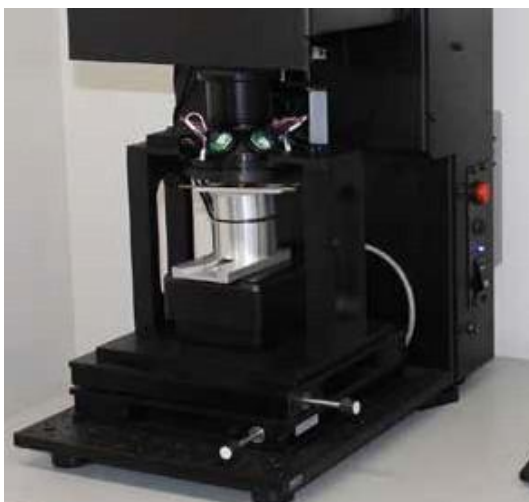
TopMatch-GS 3D Version 2 Scanner: example of photometric stereo technology
