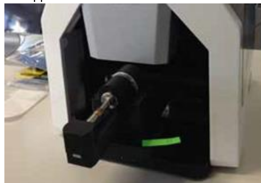
PH-5000 Interferometer microscope: example of coherence scanning interferometry technology
