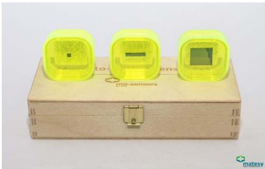
Figure 6. MO sensor kit showing the three sensor sizes used in the project.
