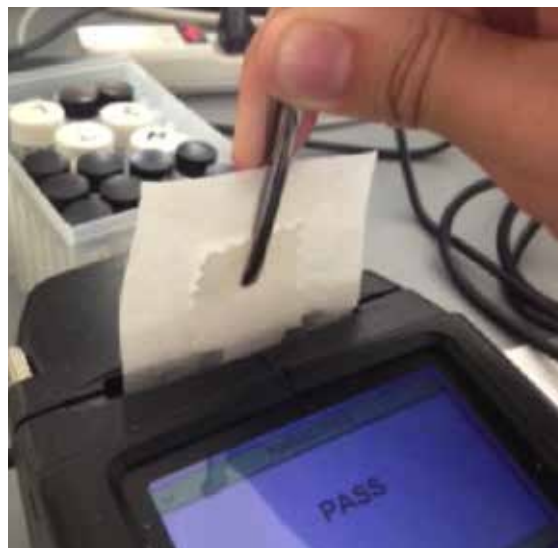
Muslin sample being inserted into Sabre ® IMS.
