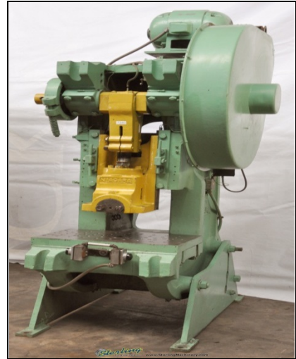
Figure 7. Open back, inclinable press used for stamping serial numbers.
