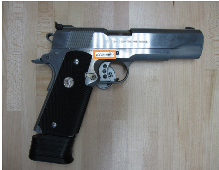
Figure 1. 45 automatic Colt with obliterated serial number on the frame.
