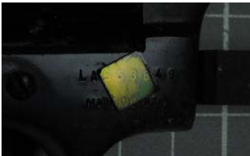
Figure 8. MO sensor methodology confirmatory step showing stamped alphanumeric characters.
