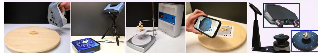
**Figure 2.** 3D scanners used. From left to right: Artec® Spider® (\$17.5K), EinScan® Pro 2X (\$6K), NextEngine® Ultra HD (\$3K), Qlone® photogrammetry (\$0), Solutionix® C500 (\$38K).
