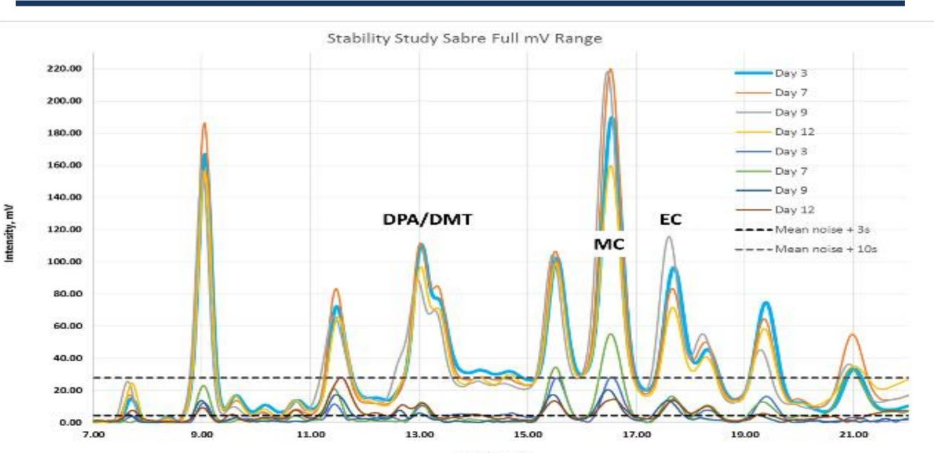
Samples stored at room temperature and exposed to room lighting. Data collected on a Smiths Detection Ionscan<sup>®</sup>.
