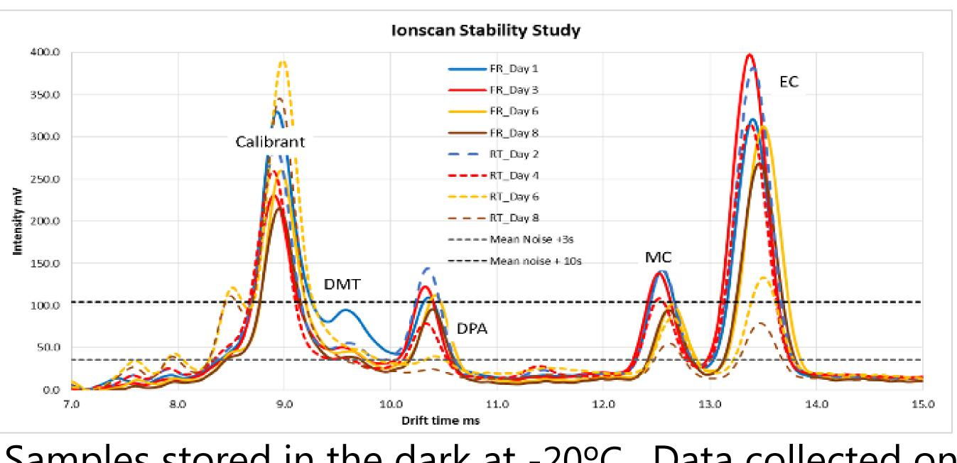
Samples stored in the dark at -20°C. Data collected on a Smiths Detection Sabre®.
