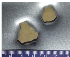
Fig 4. Holes in 22 gauge sheet metal (0.028” or 0.71mm) made by PolyCase Inceptor ARX bullets. Note triangular shape of holes. Caliber 45 ACP on left fired from Kimber 1911, 9mm L on right fired from S&W 5946.
