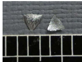
Fig 5. “Punchouts” recovered in ballistic gel from 22 gauge sheet metal perforated by PolyCase Inceptor ARX bullets.
