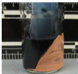
Fig 2. The components of a PolyCase Inceptor ARX bullet deconstructed, revealing copper spheres and polymer.
