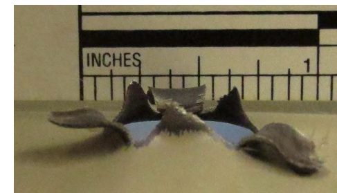
Fig 8. Side view of exit hole in 22 gauge sheet metal made by 40 S&W PolyCase ARX bullet. Note 3 sharp points and 3 peeled back petals.
