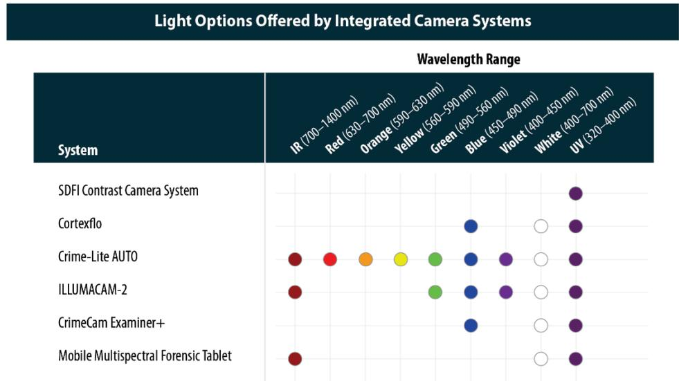
**Exhibit 8. Integrated camera systems enable SANEs to photograph using visible light, white light, ALS, UV light, and IR light techniques.** These colors represent wavelength ranges as noted in Exhibit 1 and Exhibit 6. Please note that this exhibit may not capture all specific wavelengths emitted by the integrated system (e.g., Crime-lite AUTO’s 55 wavelength combinations).
