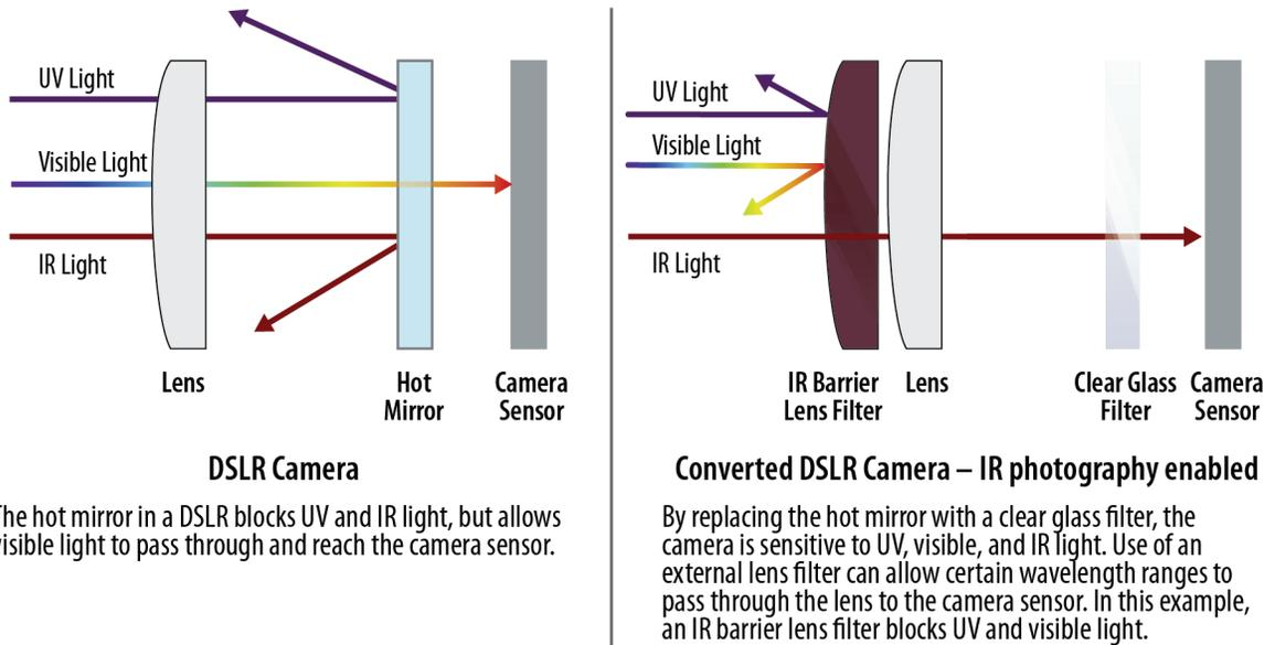
\*This representation does not accurately depict spacing of components within a camera, but is meant to show a schematic of DSLR conversion. Any UV coating present on the camera lens may lead to some UV light reflection.
