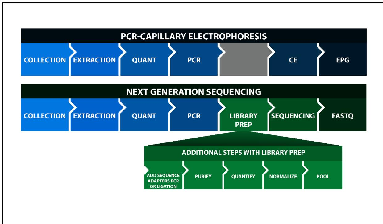
Extra steps are highlighted in the green “library prep” inset. Sequencing requires a slightly more complex procedure. Resulting data output format and analysis software are also different.
