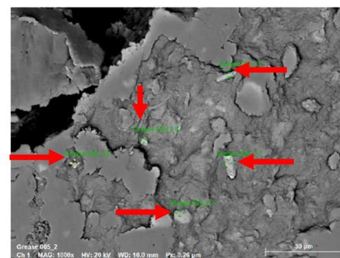
Figure 6. SEM image of grease samples. Red arrows indicate particles where measurements were taken
