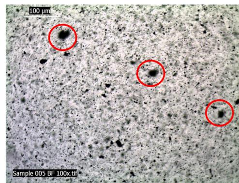
Figure 1. Microphotograph of grease sample. Red circles indicate the observed particles that were part of the original manufacturing formulation
