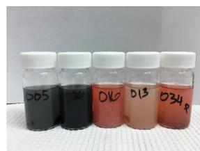
Figure 2. Five grease samples being dissolved in solvent
