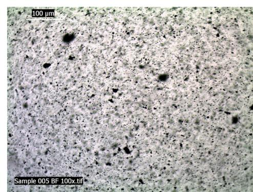
Figure 5. Microphotographs showing before and after extraction with solvent. The density of the components increased, suggesting the removal of the base oil
