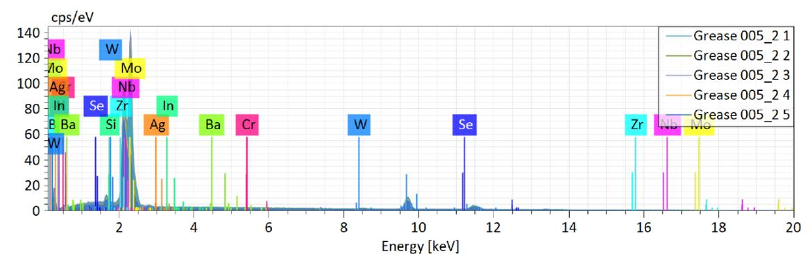
Figure 7. EDS spectrum of particles showing elemental composition of several particles within the greases. The main components found were molybdenum and niobium
