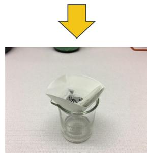
Figure 3. Gravity filtration of sample 005 using Whatman filter paper
