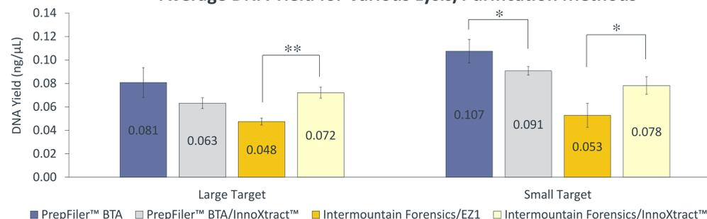
Figure 2. Average DNA Yield for Lysis methods – The coupling of InnoXtract™ purification with PrepFiler™ BTA lysis provided a higher small target yield (n.s.) compared to Intermountain Forensics lysis and InnoXtract™ purification; (Data reported as  $\mu \pm \sigma$ ; \* indicates a p-value < 0.05; \*\* indicates a p-value < 0.005).
