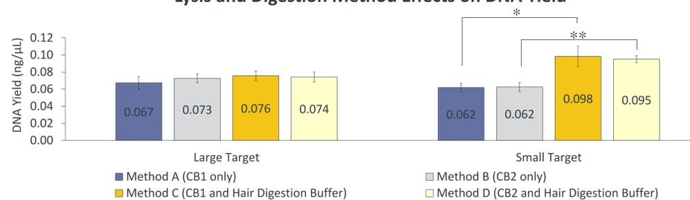
Figure 3. InnoXtract™ Lysis and Digestion Method Effects on DNA Yield – Two-part digestion resulted in a significant increase in small target DNA yield. No significant difference was seen with the addition of salt; (Data reported as  $\mu \pm \sigma$ ; \* indicates a p-value < 0.01, \*\* indicates a p-value < 0.005).
