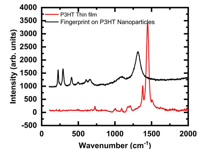
Figure 3. Raman scattering of P3HT film and fingerprint on P3HT nanoparticles
