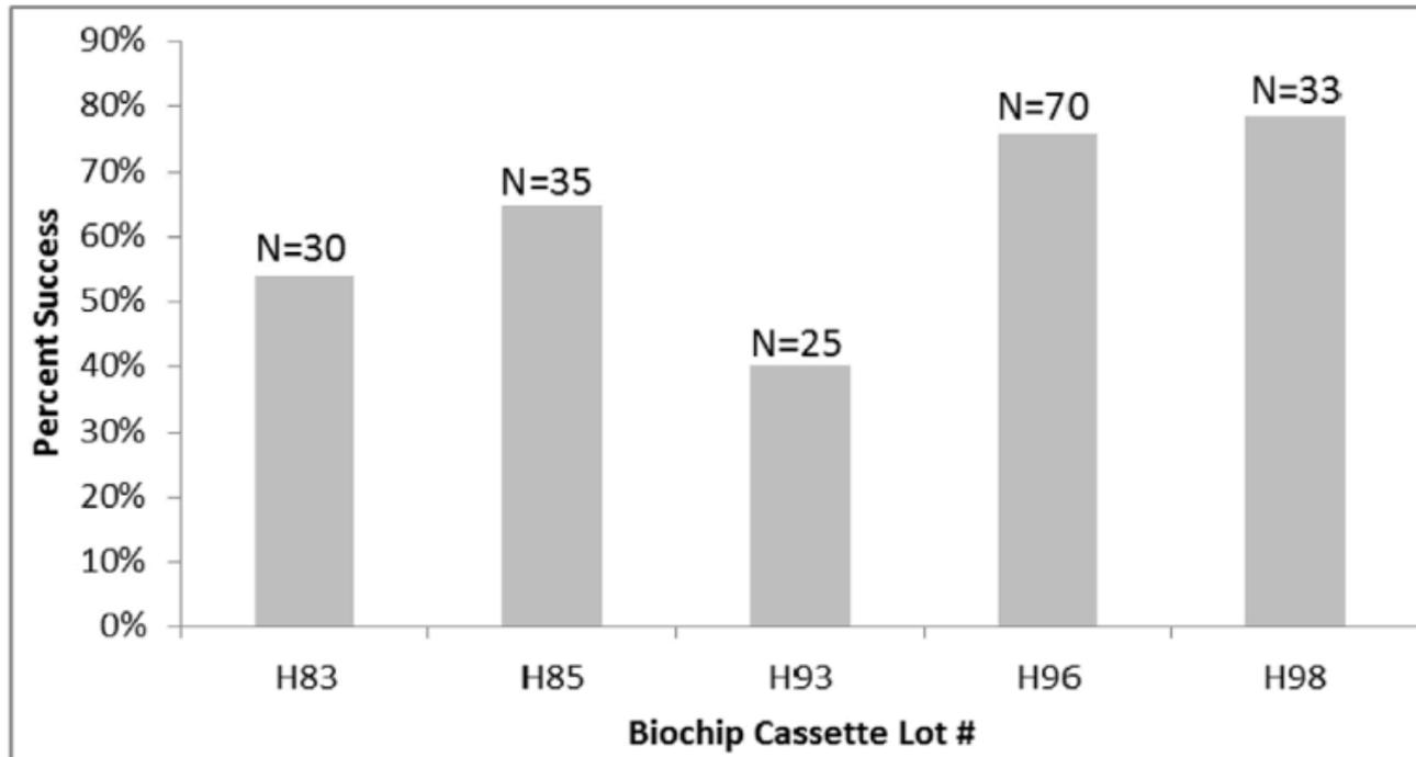
**Fig. 4.** Biochip cassette lot-to-lot comparison. The number of known samples run with each of the lots is included for reference. Four of the five lots used exhibited >50% success, but one of the lots (H93) exhibited a decreased level of success. Samples run with these lots and used in the sensitivity study were not counted as part of this evaluation.
