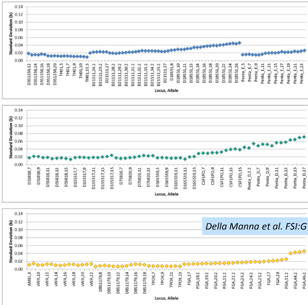
Fig. 6. Sizing variation at a single standard deviation for each allele in the allelic ladder calculated for 418 runs on 14 DNAscan instruments.
