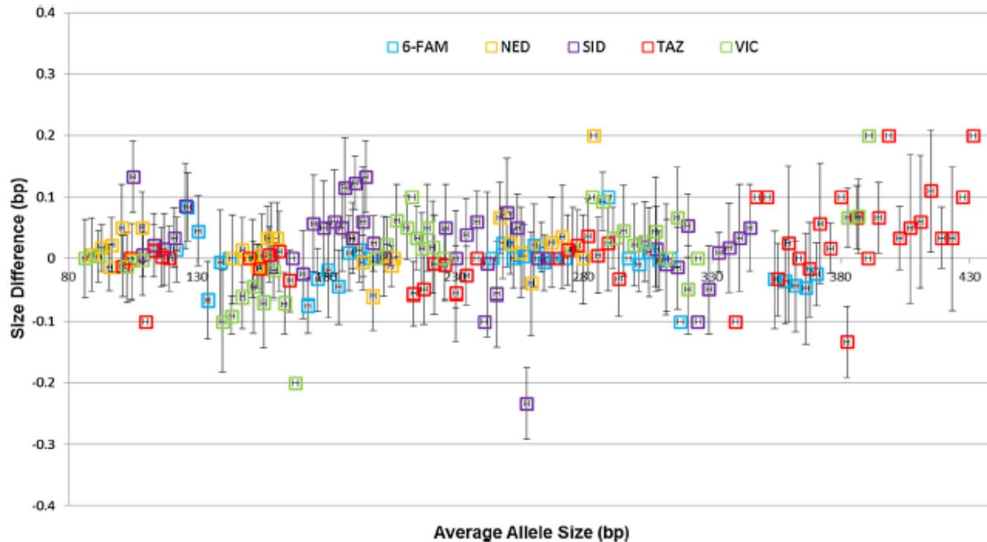
**Fig. 9.** Accuracy. Size difference (in base pairs) between an allele and its corresponding allele in the allelic ladder used to size the sample (53 samples, 2138 alleles). The color of each data point indicates the corresponding dye in the GlobalFiler<sup>®</sup> Express assay; FAM (blue), VIC (green), NED (yellow), TAZ (red) and SID (purple).
