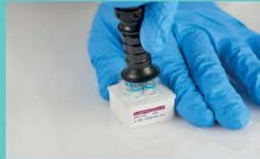
Insert collector into test plate.
