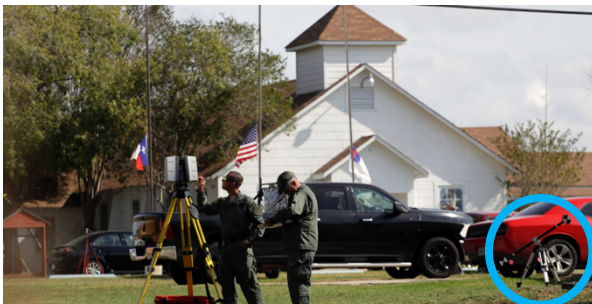
Law enforcement operating a 3D scanner at the Sutherland Springs shooting scene. A NIST calibration tool is indicated in blue. Photo credit: AP Photo (Eric Gay).
