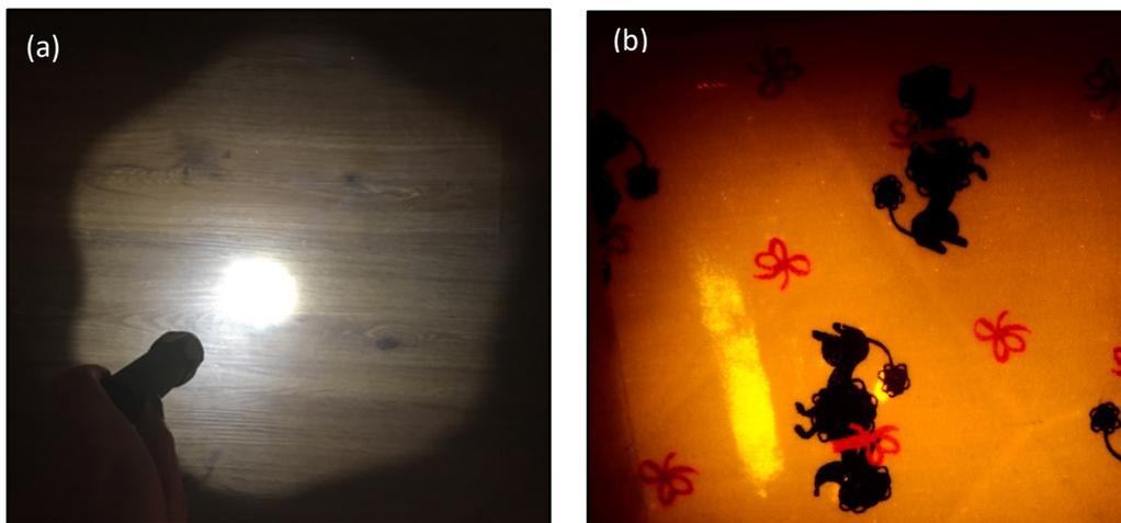
**Figure 5.** Demonstration of a hot spot (a) with a white light and (b) with a blue ALS visualized through orange barrier filter goggles. The light in the center is more intense than the surrounding light.
