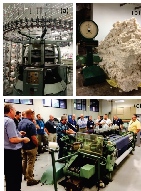
Fig. 5. (a) Jersey circular knitting machine in the knitting laboratory; (b) raw cotton in the spinning laboratory; and (c) a loom making denim in the weaving laboratory. Photo credit: RTI staff.
