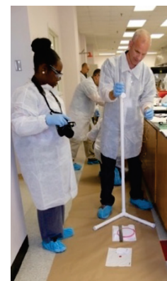
Assessing drip stains from a 90° angle onto different textile substrates. Photo credit: RTI staff.
