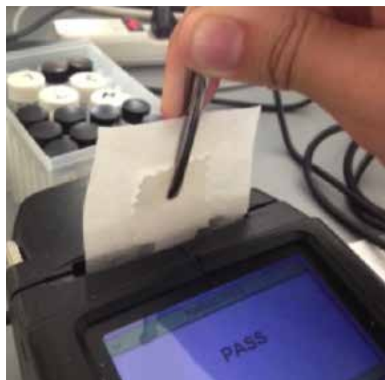
Muslin sample being inserted into Sabre ® IMS.
