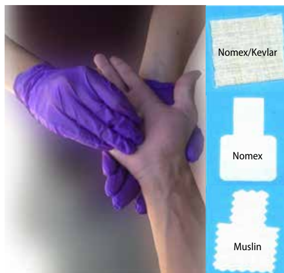
Hand swabbing and typical examples of hand swab materials Nomex/Kevlar, Nomex, and Muslin.
