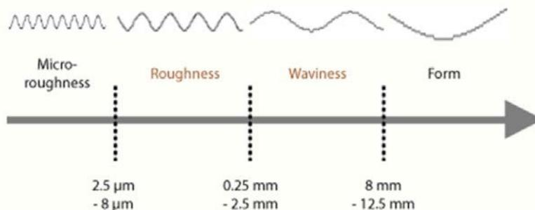
Figure 4. Four components of surface texture<sup>12</sup>
