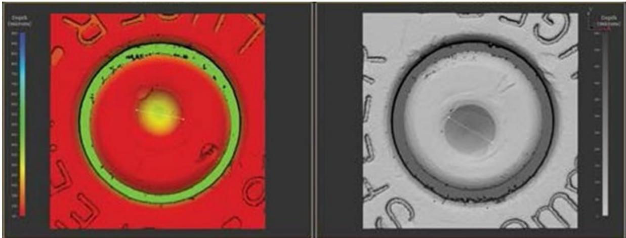
**Figure 1. Topographical image of breech face and firing pin impressions<sup>6</sup>**
