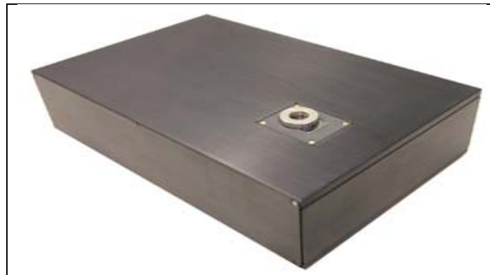
Figure 4. CMOS Magview with O-ring placed on the MO sensor (source: Matesy GmbH).
