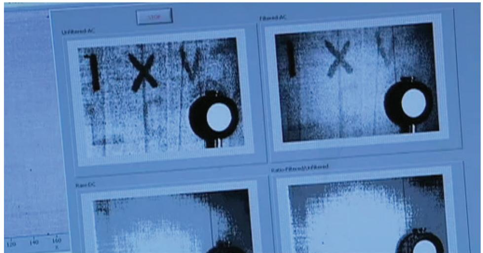
Example images of blood stains captured using the prototype IR camera that was developed with the support of NIJ funding.
